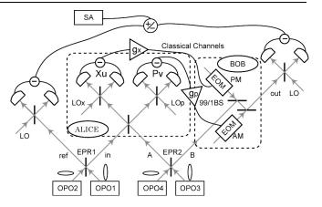
FIG. 1. The experimental setup for teleportation of quantum entanglement. OPOs are optical parametric oscillators. All beam splitters except 99/1 BSs are 50/50 beam splitters. LOs are local oscillators for homodyne detection. SA is a spectrum analyzer. The ellipses illustrate the squeezed quadrature of each beam. Symbols and abbreviations are defined in the text.
